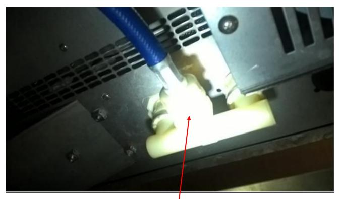
Remove the white plastic water inlet fitting before connecting the BRITA filter and separate mains water hoses
